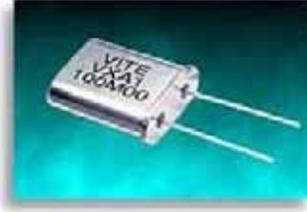
Vite's standard crystal tolerance (Option "B" under stability vs. temperature) is  $\pm 50$  PPM  $-20^{\circ}\text{C}$  to  $+70^{\circ}\text{C}$  relative to the load capacitance at  $+25^{\circ}\text{C}$ . All VXA crystals will operate  $-40^{\circ}\text{C}$  to  $+85^{\circ}\text{C}$ .
